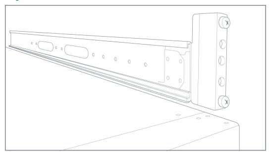
Figure 2: Slide Rail Installed in Four Post Rack
