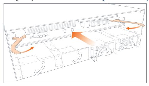
Figure 21: Control Card Ejector Handles
