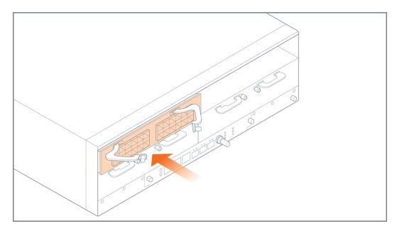
Figure 12: Module Insertion
