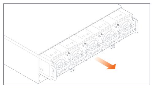
Figure 11: Fan Tray Removal
