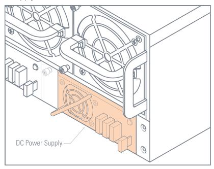
Figure 4: DC Power Supply Module
