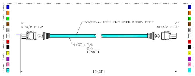
Figure 1: MPO/MTP 12 Position Fiber Cable
