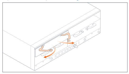
Figure 9: Filler Panel Levers
