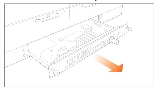
Figure 16: Extension Board Removal
