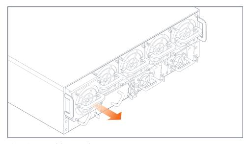
Figure 8: Fan Module Removal
