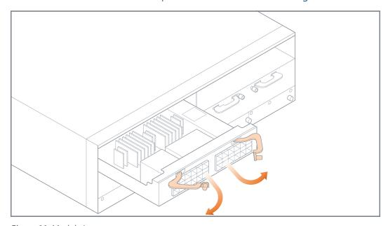
Figure 11: Module Levers
