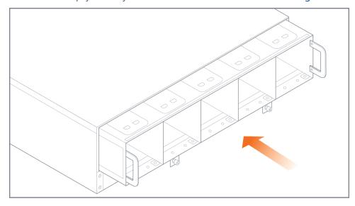
Figure 12: Fan Tray Insertion
