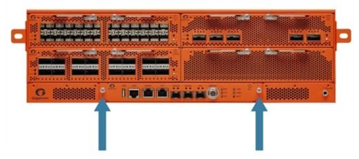
Figure 15: Extension Board Screw Location on GigaVUE-HC3 Front
