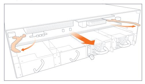
Figure 18: Control Card Ejector Handles
