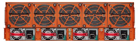
Figure 6: Four Power Supply Modules Installed
