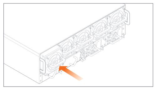
Figure 9: Fan Module Insertion
