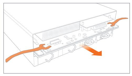
Figure 19: Control Card Removal
