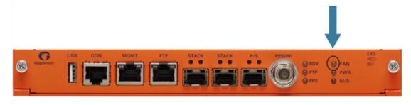
Figure 5: Global Fan LED Location on GigaVUE-HC3 Front
