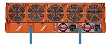
Figure 10: Fan Tray Screw Location on GigaVUE-HC3 Rear
