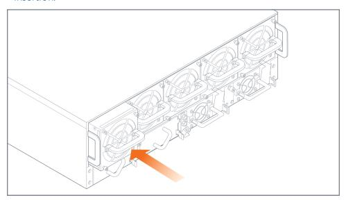
Figure 14: Fan Module Insertion
